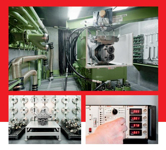
Due to a wide range of custom adaptations, we are capable of testing virtually 100% of all hydraulic pumps and motors available on the market using our test bench.
